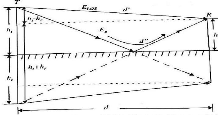
The method of images is used to find the path difference between the line-of-sight and the ground reflected paths.
