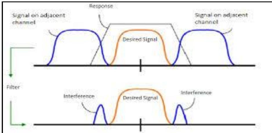
**Adjacent-channel interference (ACI)** is interference caused by extraneous power from a signal in an adjacent channel. ACI may be caused by inadequate filtering, improper tuning or poor frequency control (in the reference channel, the interfering channel or both).
