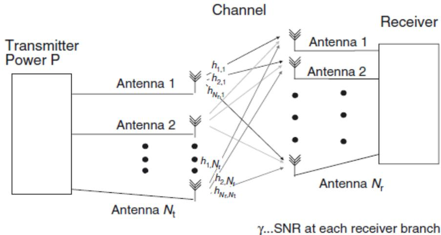
Figure Block diagram of a multiple-input multiple-output system.
