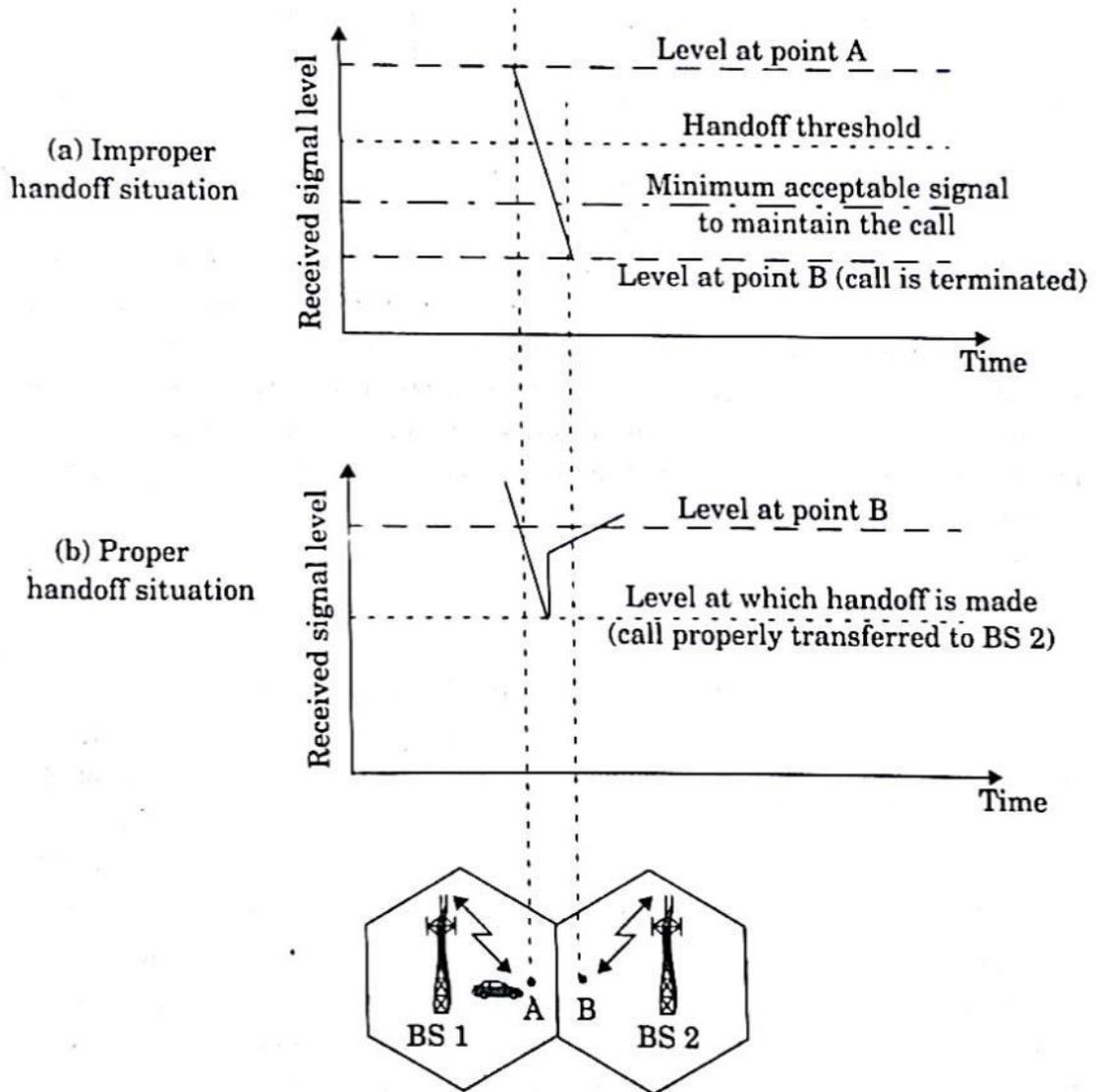
Fig: Illustration of a handoff scenario at cell boundary
