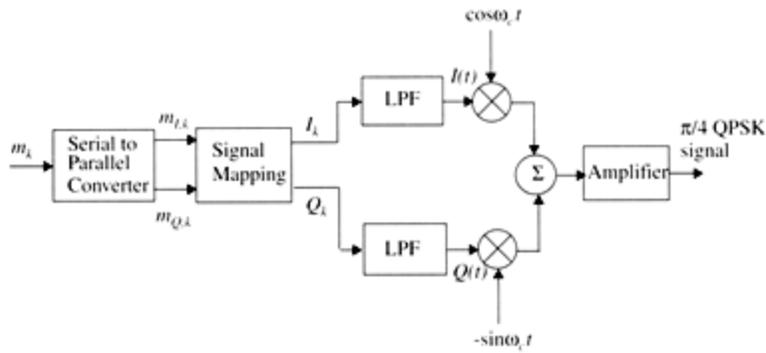
Figure Generic  $\pi/4$  QPSK transmitter.
