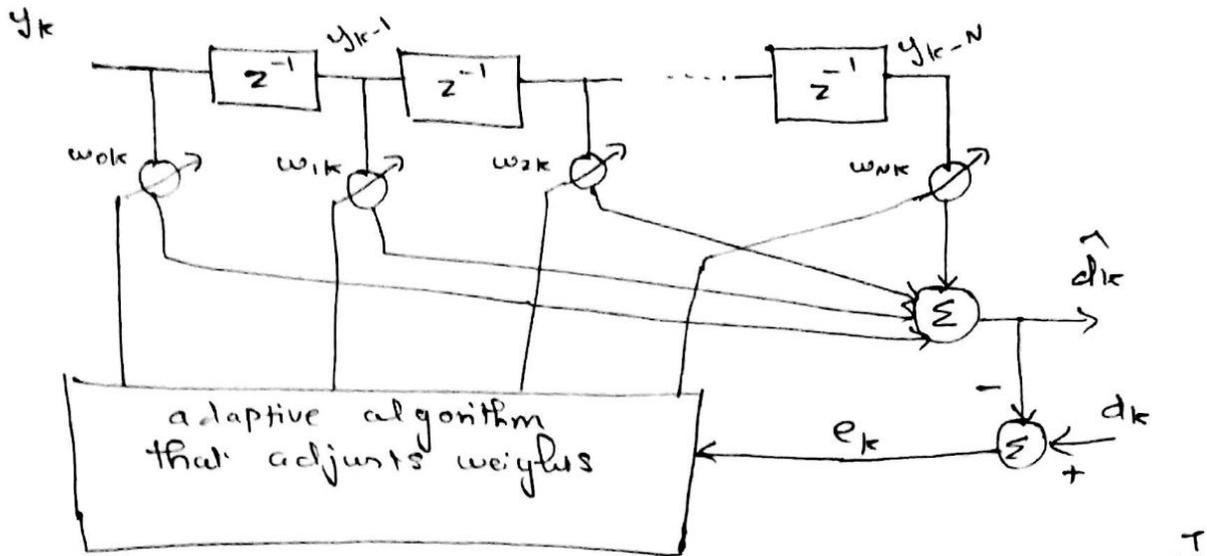
Input to the equalizer  $y_k = [y_k, y_{k-1}, y_{k-2}, \dots, y_{k-N}]^T$
