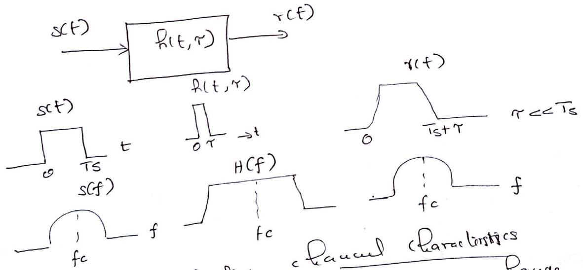
flat fading channel characteristics
