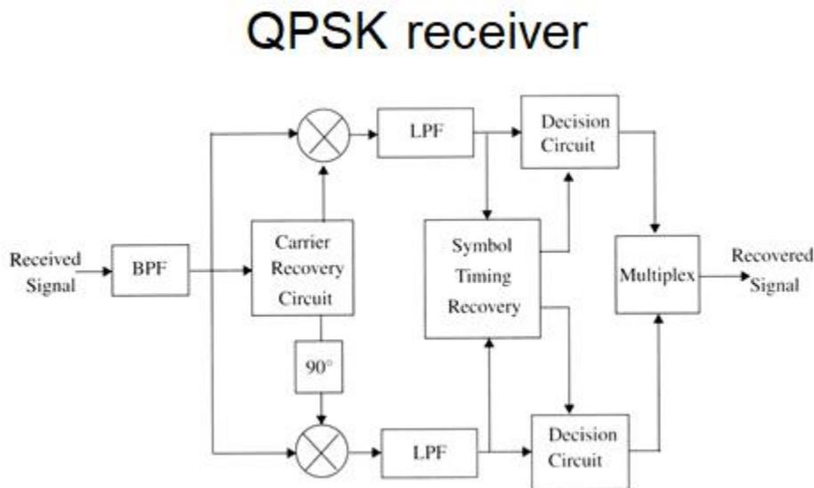
**Figure** Block diagram of a QPSK receiver.
