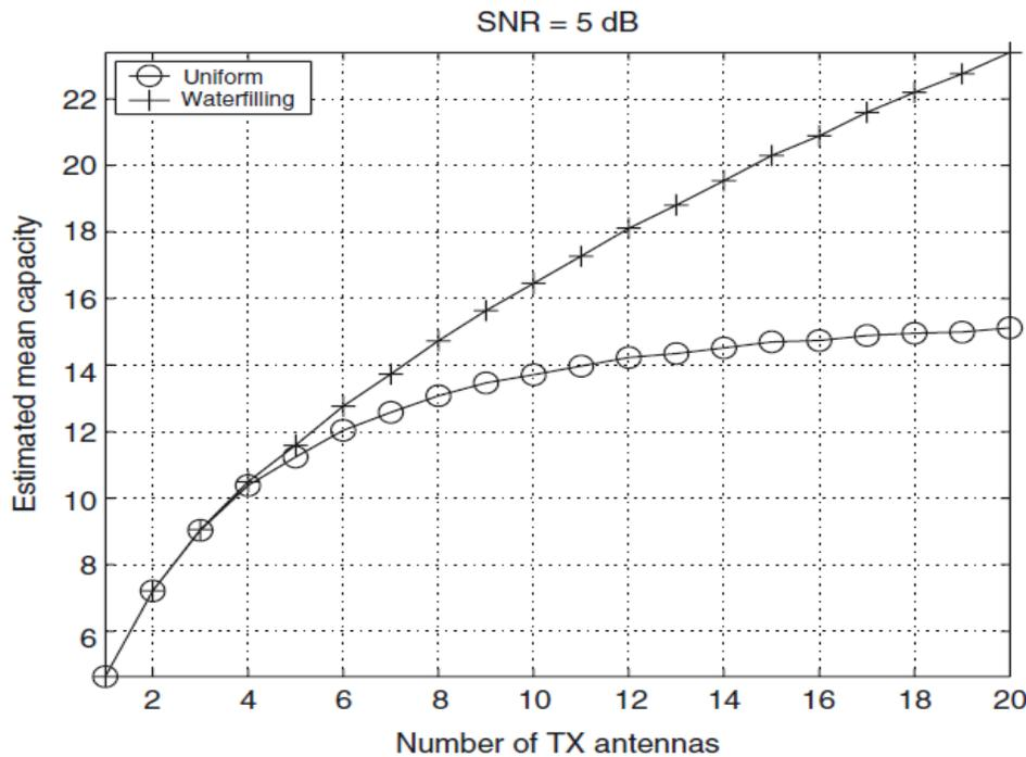
**Figure** Capacity with and without channel state information at the transmitter with  $N_r = 8$  antennas and a signal-to-noise ratio of 5 dB.
