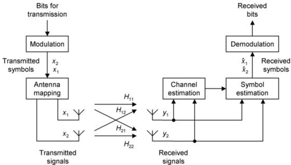
**Basic principle of a 2x2 spatial multiplexing system**
