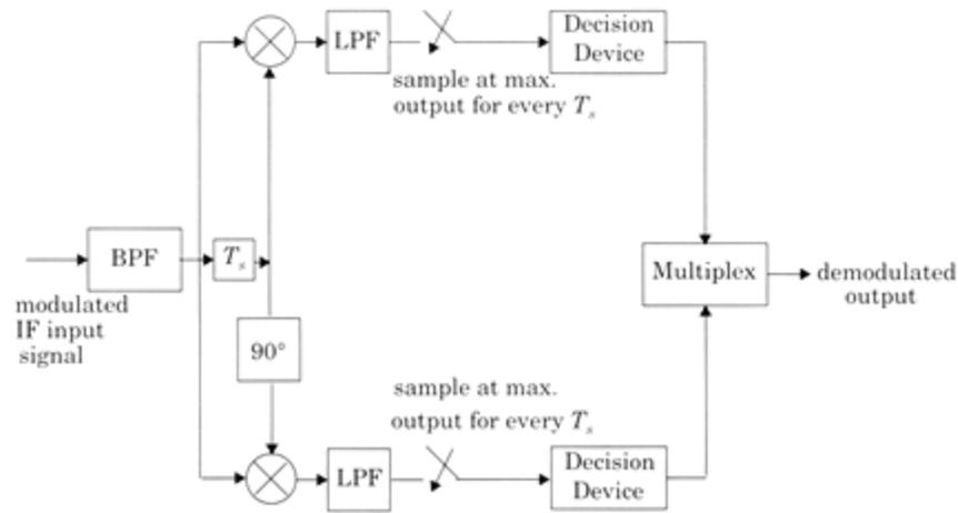
Figure . Block diagram of an IF differential detector for  $\pi/4$  QPSK.
