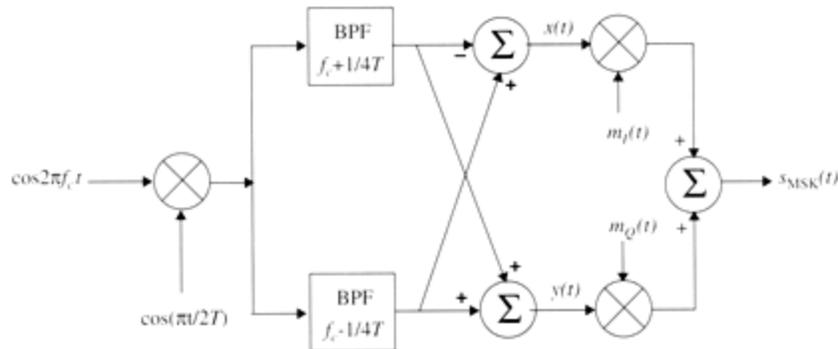
Figure Block diagram of an MSK transmitter. Note that  $m_I(t)$  and  $m_Q(t)$  are offset by  $T_b$ .
