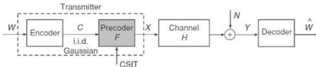
**Precoding for point – to – point MIMO systems**
