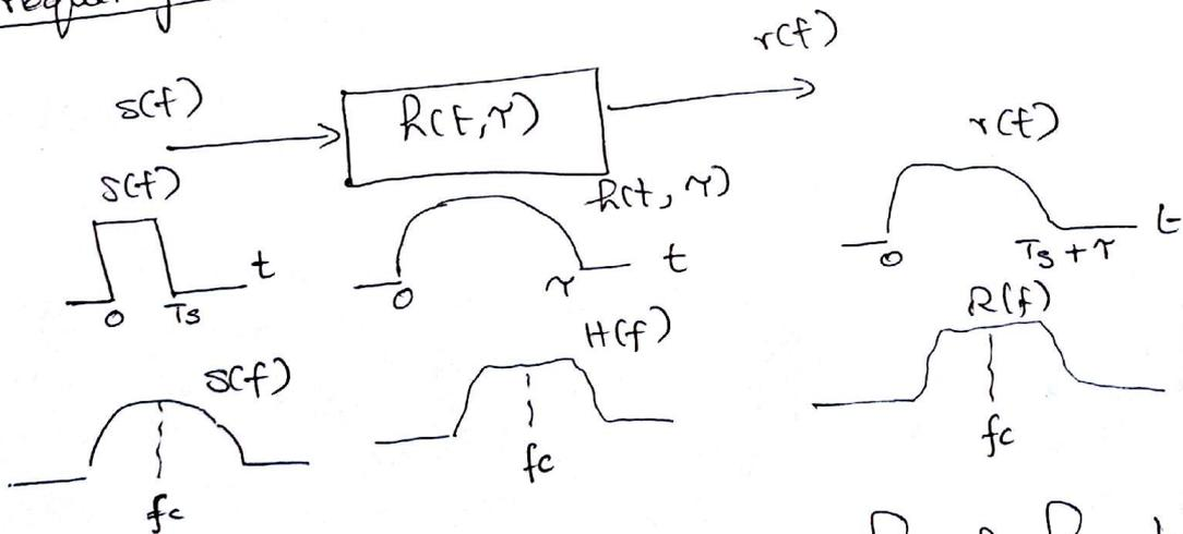
frequency selective fading statistics channel characteristics.
