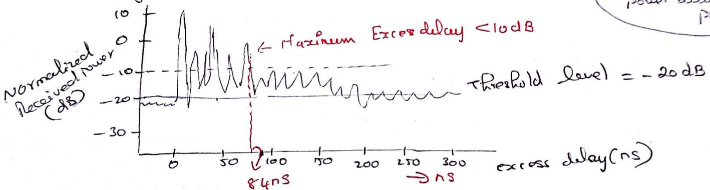
values for  $\bar{\tau}$ ,  $\bar{\tau}^2$  and  $\sigma_\tau$  depend on the choice of noise threshold used to process  $P(\tau)$
