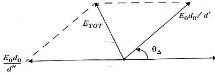
Phasor diagram showing the electric field components of the line-of-sight, ground reflected, and total received E-fields
