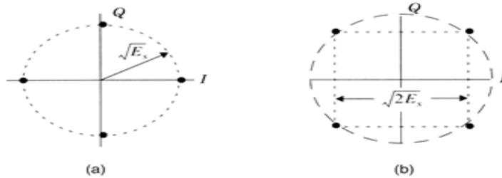
**Figure** (a) QPSK constellation where the carrier phases are  $0, \pi/2, \pi, 3\pi/2$ ; (b) QPSK constellation where the carrier phases are  $\pi/4, 3\pi/4, 5\pi/4, 7\pi/4$ .
