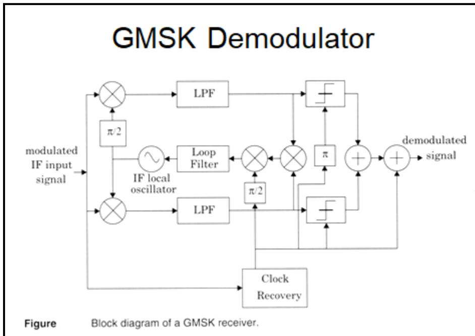
Figure Block diagram of a GMSK receiver.
