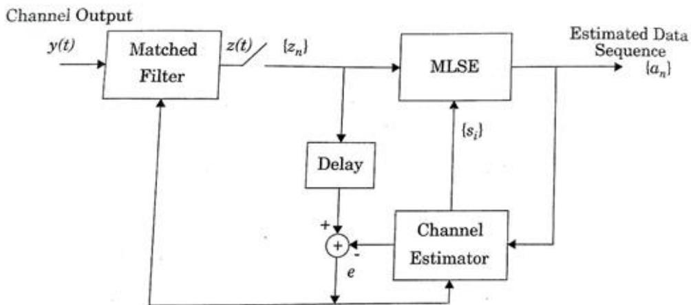
Figure The structure of a maximum likelihood sequence estimator (MLSE) with an adaptive matched filter.
