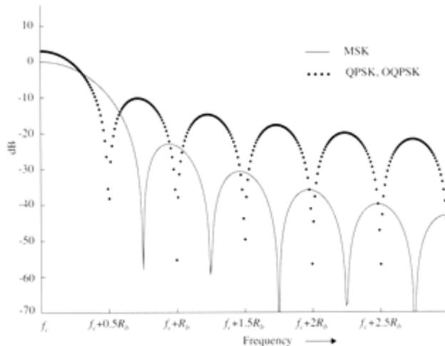
Figure Power spectral density of MSK signals as compared to QPSK and OQPSK signals.
