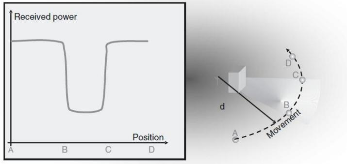
The principle of shadowing.
