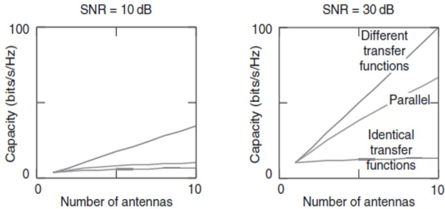
Figure . Capacity of multiple-input-multiple-output systems in additive white Gaussian noise channels.
