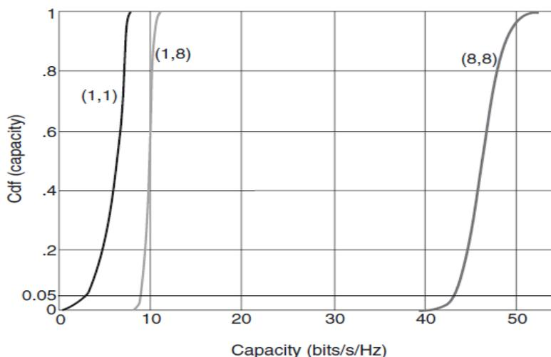
**Figure** . Cumulative distribution function of capacity for  $1 \times 1$ ,  $1 \times 8$ , and the  $8 \times 8$  optimum scheme.
