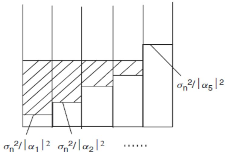
**Figure** Principle behind waterfilling.
