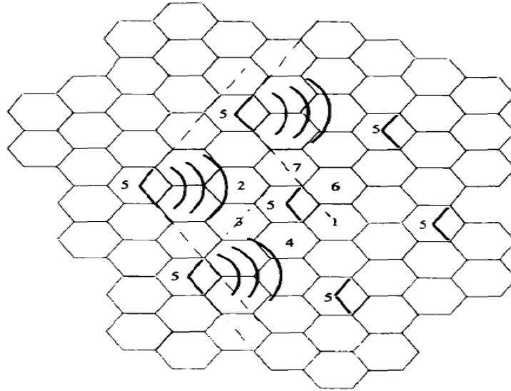
**Illustration of how 120° sectoring reduces interference from co-channel cells. Out of the 6 co-channel cells in the first tier, only 2 of them interfere with the center cell. If omni-directional antennas were used at each base station, all 6 co-channel cells would interfere with the center cell.**
