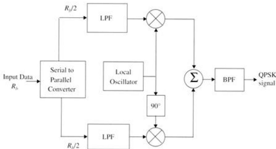
**Figure** Block diagram of a QPSK transmitter.
