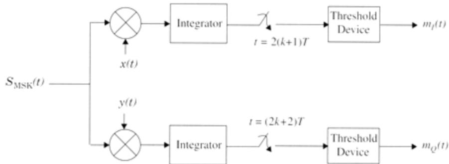
Figure Block diagram of an MSK receiver.
