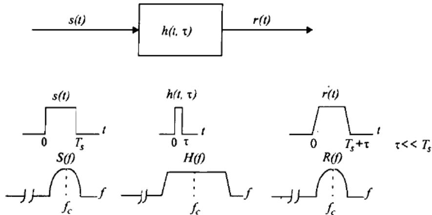
**Flat fading channel characteristics.**
