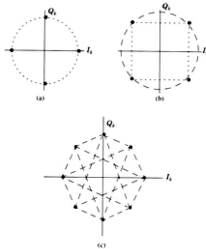
Figure Constellation diagram of a  $\pi/4$  QPSK signal: (a) possible states for  $\theta_k$  when  $\theta_{k-1} = n\pi/4$ ; (b) possible states when  $\theta_{k-1} = n\pi/2$ ; (c) all possible states.
