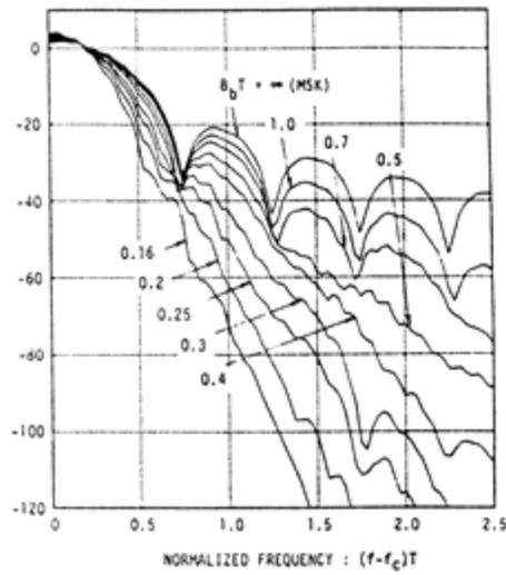
Figure Power spectral density of a GMSK signal [from [Mur81] © IEEE].
